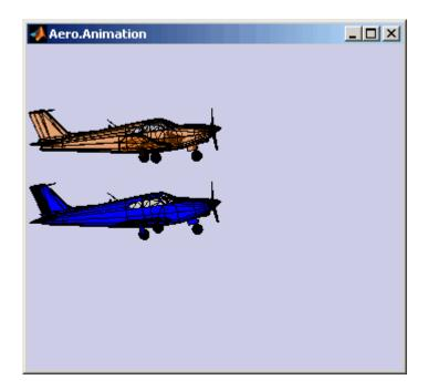
**Changing the Color of the Second Body.** This series of commands illustrates how to change the color of a body. The animation object stores the body geometry as patches. This example will manipulate the FaceVertexColorData property of these patches.
